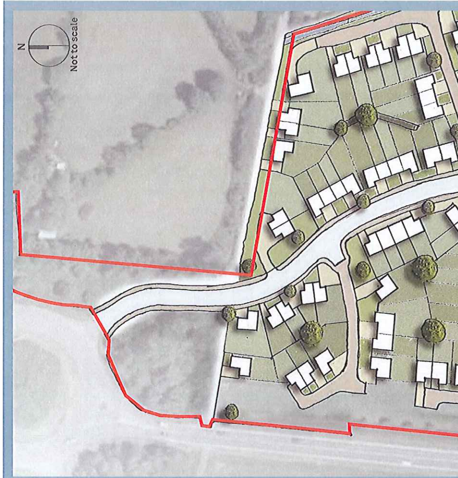
Extract from illustrative layout plan demonstrating how the access road shown to the left could be feasibly integrated into an attractive development proposition.
